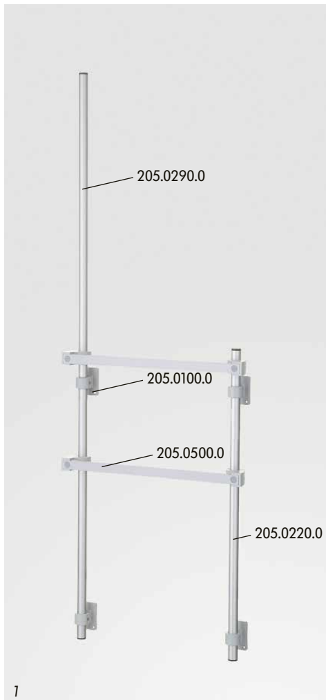
1 Rack for supporting accessories 205.4000.0 aluminium/plastic, lateral mounting to functional trolley, comprises: 4 pc Basic fastening elements (205.0100.0) 1 pc Main tube 1,500 mm (205.0290.0) 1 pc Main tube 800 mm (205.0220.0) 2 pc Accessory rails 25 x 10 x 510 mm (205.0500.0)
